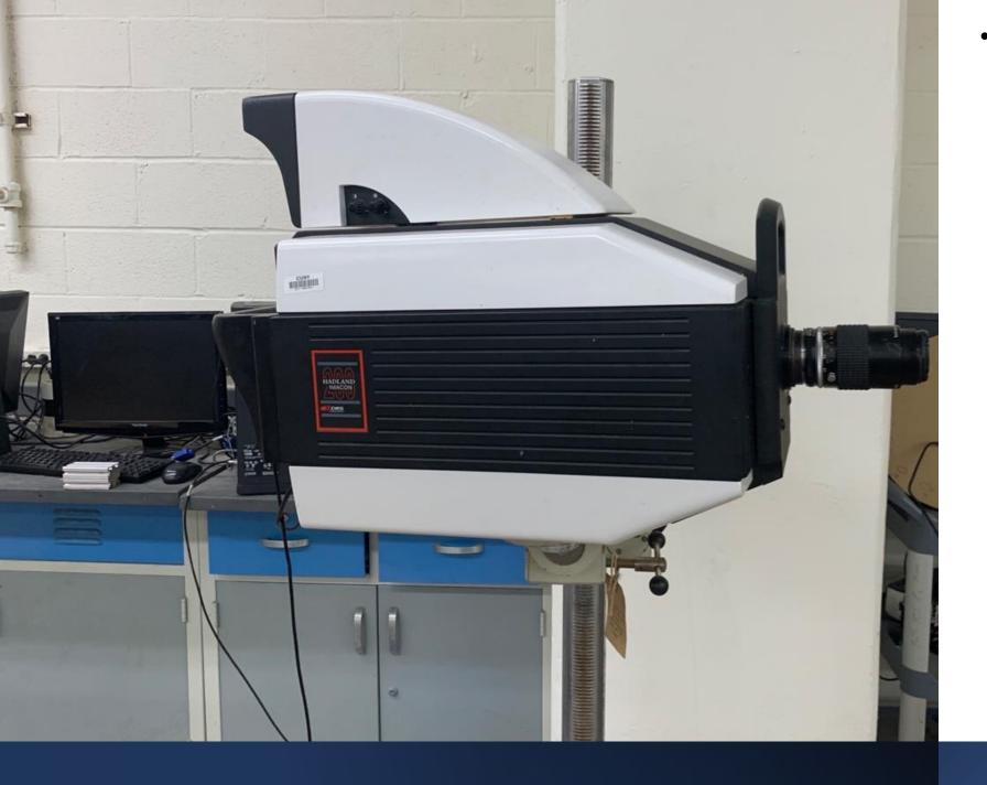
High speed camera we will be using in order to record the Schlieren image of collision. This camera can capture up to 200 million frames per second!! Although this insane speed isn't necessary for our experiment, we might require around 200,000 fps.
