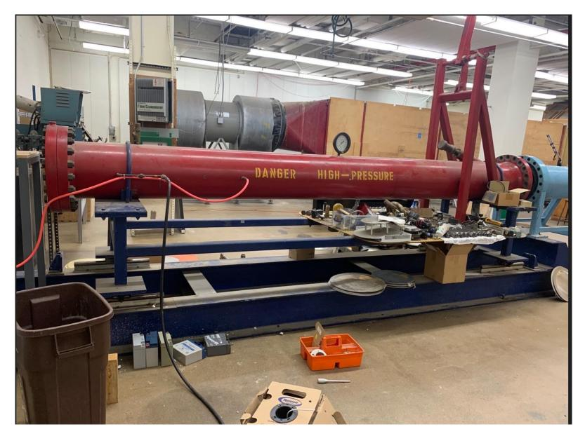
Pressure Chamber: This chamber is designed to accommodate up to 2000 PSI of pressure!!
