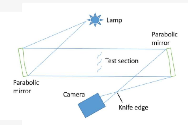
Z-Type Schlieren imaging will be used to see the fluid movement in the observation window. This imaging uses the refractive index based on different densities of fluids to visualize airflow.
